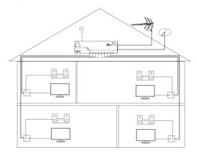
It is also suitable for upgrading or replacing existing UHF/VHF signal distribution units, simply reconnect the existing connector from the previous unit to the AMD amplifier. Ensure the UHF aerial is connected to the UHF input of the amplifier and FM/DAB aerials are connected to the VHF input of the amplifier. For loft distribution installation please ensure the unit is kept away from moisture and water.
